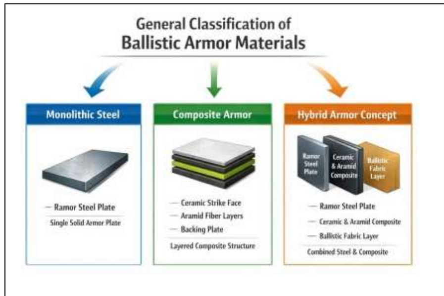
Figure 1. General Classification of ballistic armor material (monolithic steel, composite, hybrid armor concept).
